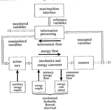
Identify the actuators, sensors, and information processing. Also provide an idea for a possible man/machine interface. (7 points)
